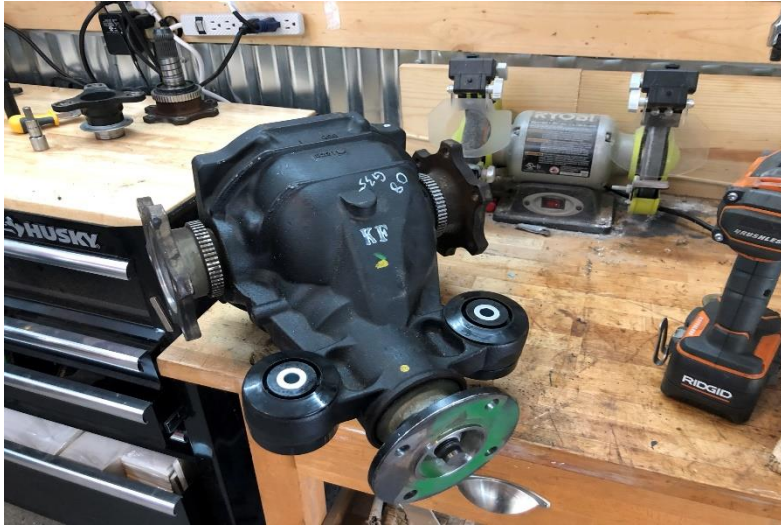
Converted G35 to Pathfinder R200 Differential
