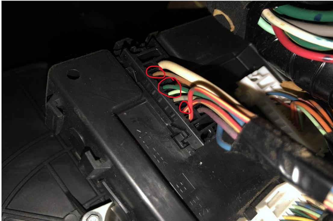
\*The BCM is located underneath the kick panel and above the gas pedal\*
